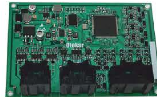
EV High Voltage Control Unit
