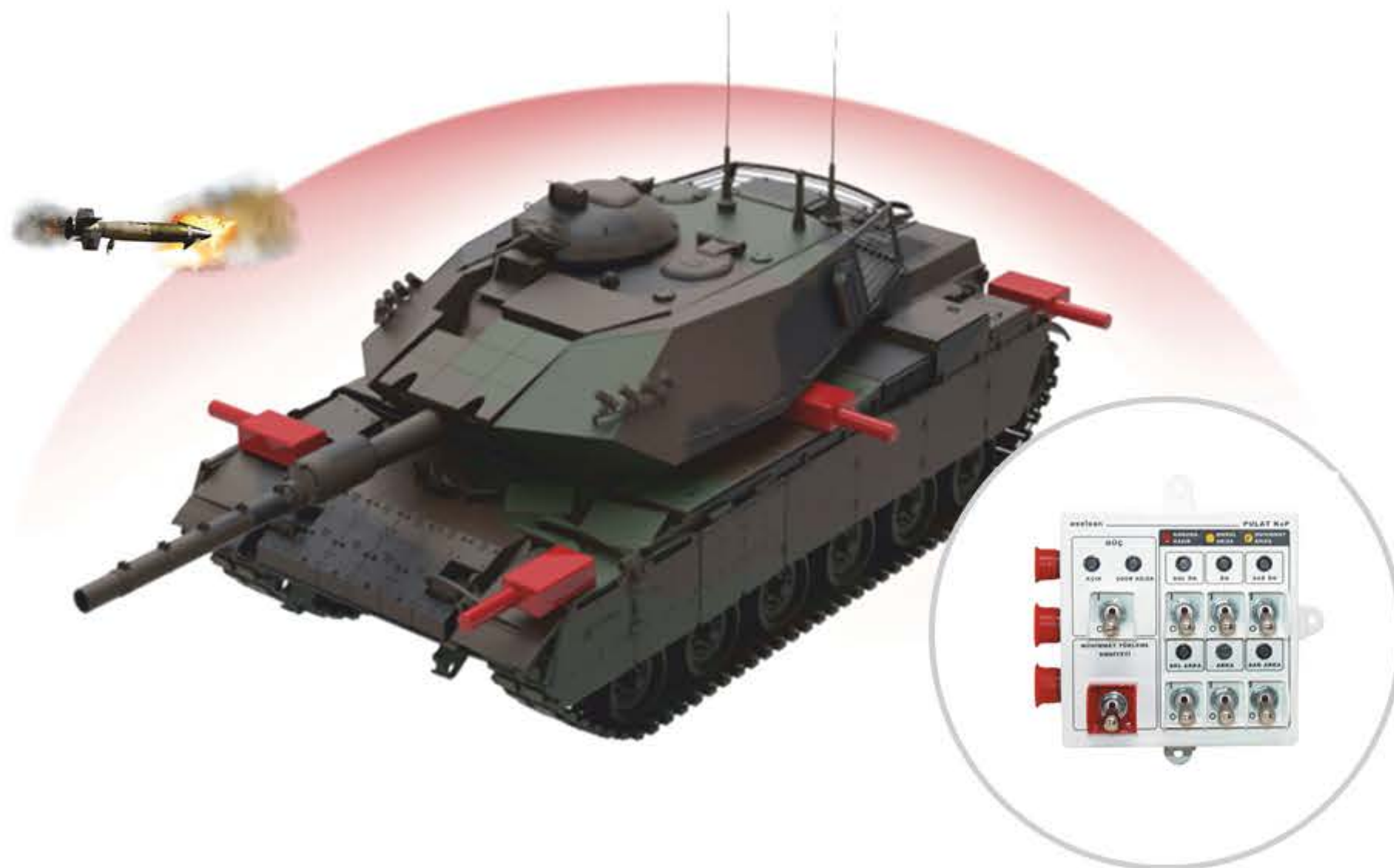
Pulat Active Protection System Control Panel
